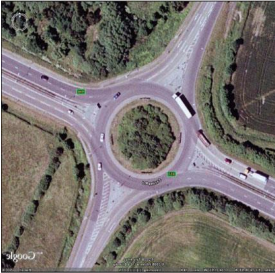
Figure 4.20: Roundabout Configuration Example
